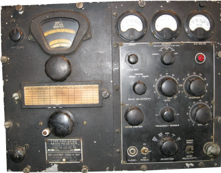
US Navy Model "RCH" – CZC-46209. Communications receiver made by E.H. Scott for the US Navy. Robert Rule, Augusta, ME.
